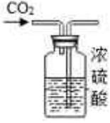
干燥CO<sub>2</sub>      B.
